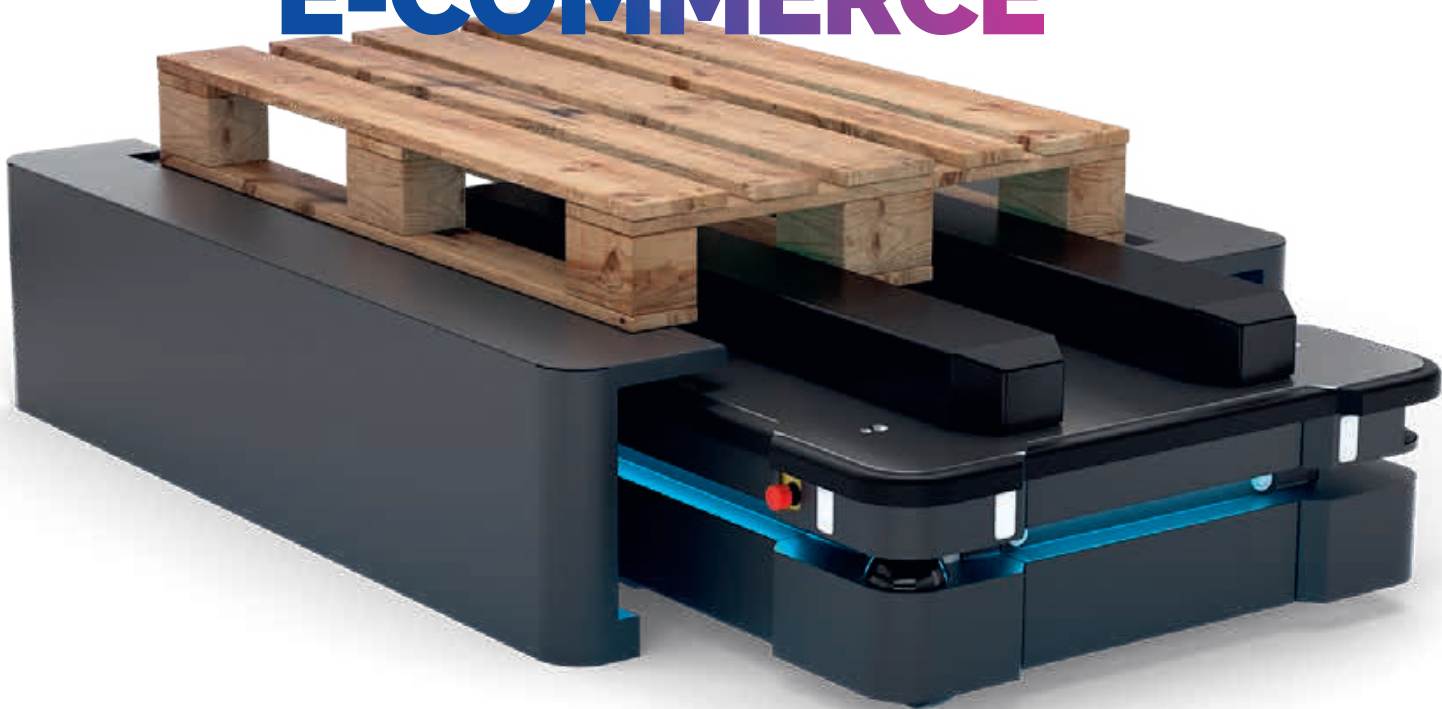
MIR 500. A collaborative robot tested in Jarosty, Poland, to carry out empty pallets.
